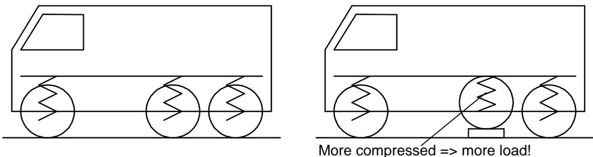
The harder the spring of the suspension the higher the effect. In the case of a rear axle of a truck a rough calculation shows that per mm compression the load rises by approximately 100 kg (Assumption: empty truck: 2t axle load; fully loaded: 12t; difference 10t; compression of the suspension unloaded to fully loaded: 100 mm; Spring rate: 10.000kg/100mm = 100 kg/mm).
