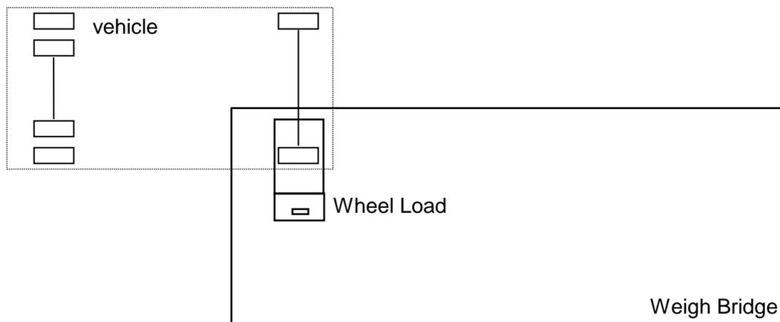
The weigh bridge has to be tarred with the Wheel Load Scale, or the weight of the Wheel Load Scale must be deducted from the indication of the weigh bridge.
